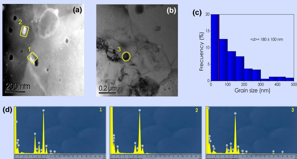
TEM images, composition and size distribution of precipitates of the ODS Fe<sub>2</sub>Y after heat treatment. (a) Ti-rich and Al-rich precipitates (b) Ti-Y-rich precipitates (c) Size distribution (d) Precipitate composition.
