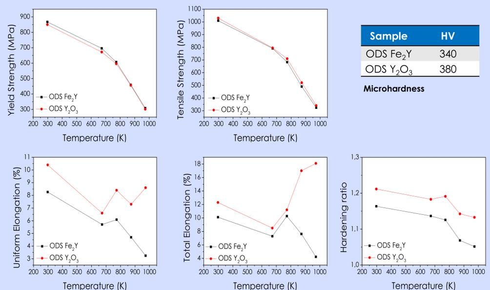
Tensile properties as a function of temperature for the ODS Fe<sub>2</sub>Y and ODS Y<sub>2</sub>O<sub>3</sub>.
