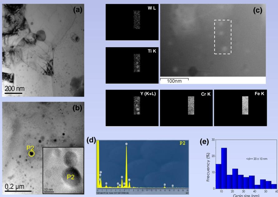
TEM images, composition and size distribution of nanoparticles of the ODS Fe<sub>2</sub>Y after heat treatment. (a) BF low magnification image showing the dispersion of nanoparticles; (b) BF image of Ti-Y-rich nanoparticles, and in-set is HREM image of the particle circled in yellow; (c) XEDS maps of nanoparticles; (d) Nanoparticle composition; (e) Size distribution.
