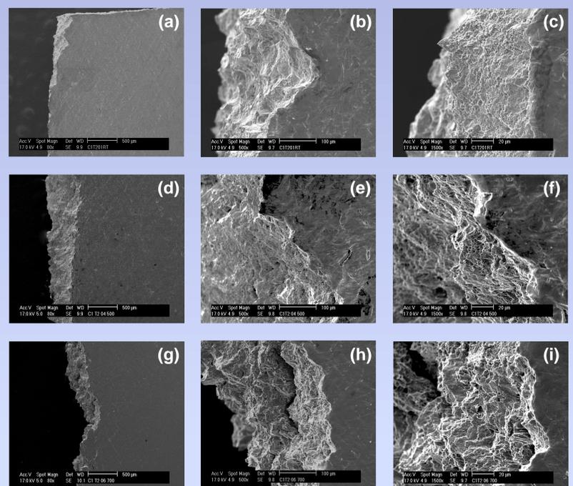
SEM fractographs showing ductile fractures in ODS Fe<sub>2</sub>Y at (a, b and c) Room Temperature, (d, e and f) 773 K and (g, h and i) 973 K
